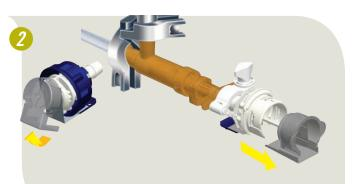
Remove the protective dust cap from the AseptiQuik STC and AseptiQuik Insert.
