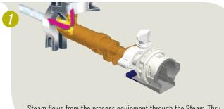
Steam flows from the process equipment through the Steam-Thru II in a steam trap creating a "steam on" sterile connection.
