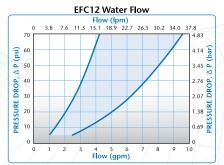
These graphs are intended to give you a general idea of the performance capabilities of each product line. The shaded area of each graph represents the operating range of the product family, i.e., upper and lower values are shown. Therefore, depending on the exact coupling configurations selected, you can reasonably expect values to fall within the shaded area.
