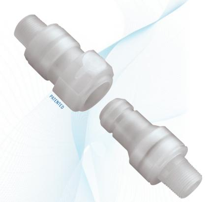
**The CQG06 Series** high purity couplings feature our patented pressurebalanced, non-spill design. Molded virgin polypropylene and a 100% springles ow path provide broad chemical resistance and exceptionally high flow capacity, allowing instant disconnects (and reconnects), even under pressure.
