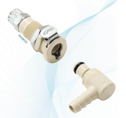
**The 1/8" flow polypropylene PMC12** offers many of the same c guration options as the PMC. The polypropylene material adds greater chemical resistance and is gamma sterilizable. The PMC12 also mates to small diameter rigid tubing. Available with a 1/4-2 at bottom port and 1/4-28 UNF threads, these couplings eliminate the need to thread and re-thread common compression nuts each time a tubing connection is made.
