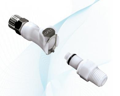
**The 1/4" flow PLC Series** is proven worldwide in thousands of applications and offers the widest selection of sizes and c gurations. PLC couplings are injection molded from acetal thermoplastic and are resistant to most mild chemical solutions. One-hand connection/disconnection, plus integral terminations make the PLC Series the choice for ease of use and manufacture.
