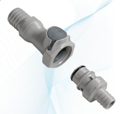
**HFC12 Series couplings** hav ow comparable to many 1/2 ow couplings in a 3/8" body size. Compact and lightweight, HFC couplings replace bulky and heavy brass ball-and-sleeve couplings in a wide range of applications. An ergonomic design and a large, shrouded thumb latch pad produce a coupling that is easy to grip and simple to operate. An efficient valve design leads to high flow and low spillage.
