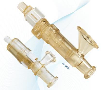
**Steam-Thru Connections** allow a quick and easy sterile connection between stainless steel biopharmaceutical processing equipment and disposable bag and tube assemblies. The single-use design saves time and money by eliminating unnecessary cleaning procedures and reducing validation burden associated with reusable components.
