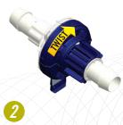
Twist the blue lock ring clockwise (approximately 75°) until audible "CPC Click" is heard. Alignment of the small blue lock ring rib indicator with the white body's rib indicator confirms final rotation is complete. Snap the membrane pull tabs together and pull from connector.
