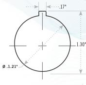
Gasket Thickness: .06\* Mounting Hole: 1.21\* diameter Coupling Spacing: 1.92\* minimum Panel Thickness: .25\*
