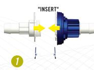
Align male and female connectors using the START alignment feature of the blue lock ring with the rib indicator of the white body. Insert the two halves together.
