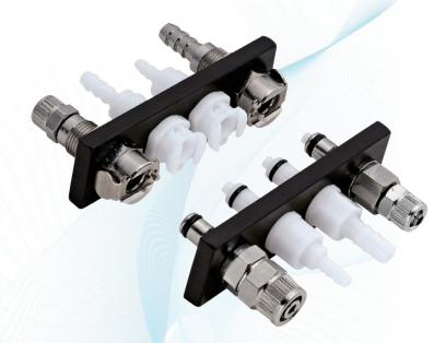
**Multi-Mount couplings** provide one easy-to-use coupling for connecting from three t ve lines at once. Multi-mount couplings are available in a wide variety of materials including acetal and chrome-plated brass. Multi-mounts are keyed to prevent mismatched connections and can be configured with or without valves for maximum design flexibility.
