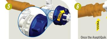
Twist the blue lock ring clockwise until audible "CPC Click." Alignment of the lock ring rib with the body's arrow indicator confirms final connection.
