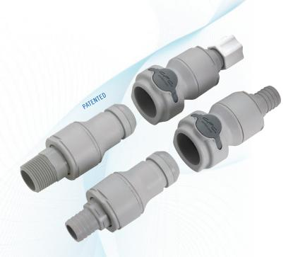
**NSH Series couplings** couplings are general purpose versions of our pressure-balanced, non-spill, ChemQuik® CQG06 couplings. Molded polypropylene, EPDM seals and a 100% springless and metal-fre ow path provide broad chemical resistance and exceptionally high flow capacity, allowing instant disconnects (and reconnects), even under pressure. Their non-spill design virtually eliminates spills, minimizes downtime and enhances operator safety in a very low cost package.
