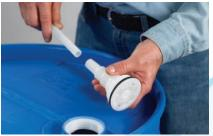
Fully press dip-tube into drum insert socket.
